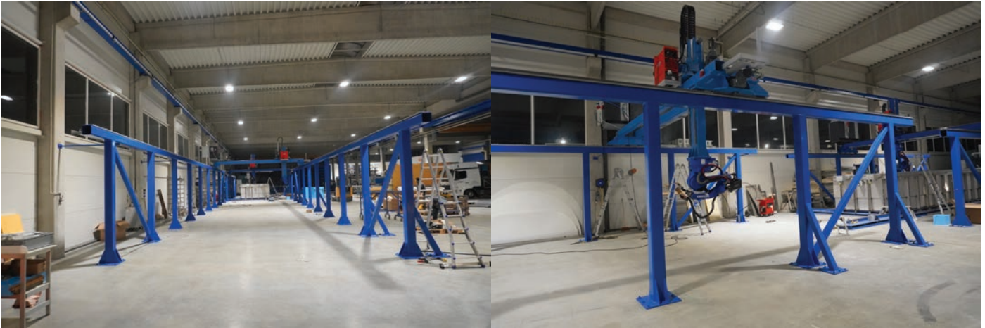
PORTAL CONSTRUCTION (26 m X axis travel, 7 m width)
