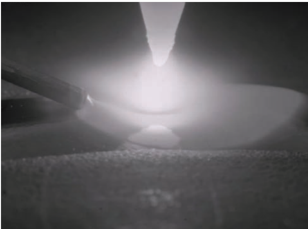
TIG (GTAW) WELDING WITH WIRE
